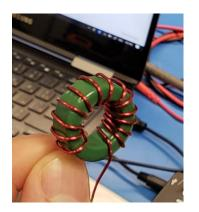
I made a 460 uH inductor (measured). Measured copper resistance is 0.16R.
