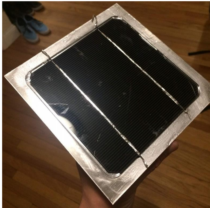
Figure 34 - Single-cell solar panel prototype with the PDMS and acrylic layers.
