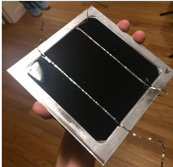
Figure 31 - Test prototype with an aluminum backplate.
