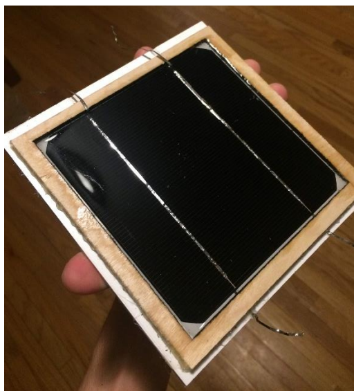
Figure 29 - PDMS-coated single-cell solar panel prototype
