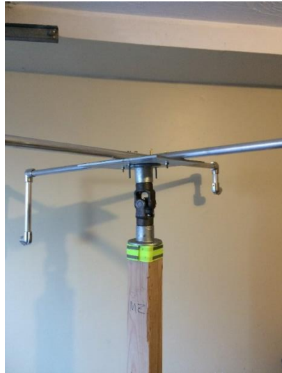
Figure 58 - Lever arms connected to a U-joint.
