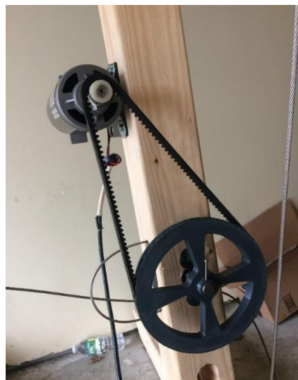
Figure 57 - 3D printed torque increasing sprocket pair connected with a rubber belt.
