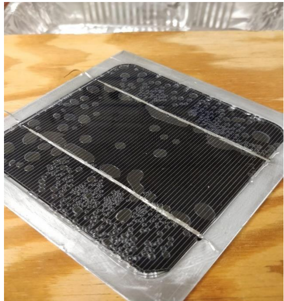
Figure 33 - Aggressive bubbling due to curing under high temperatures
